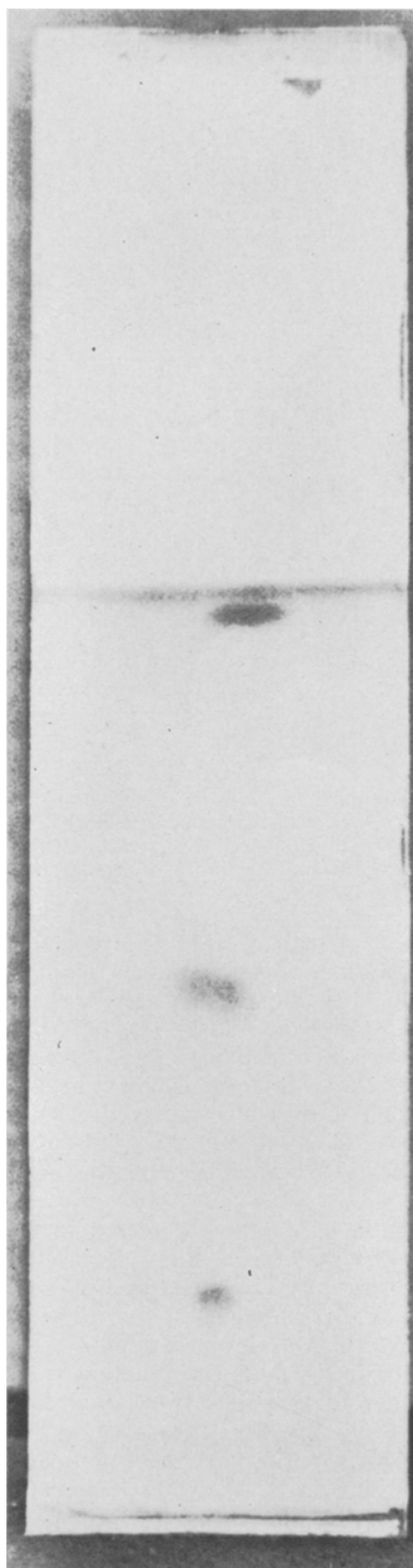
Fig. 2. Photograph of chromatographic plate, showing the separation of mono-, di-, and tripalmitin, lower, central, and upper spots, respectively.
